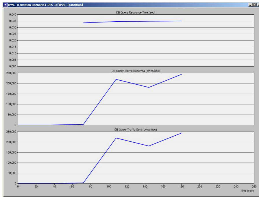
Fig. 2 Database Query Performance and Traffic of Dual Stack (Source: Researcher’s OPNET simulation results)
