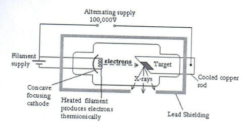
Describe how the X-rays are produced by the set up and highlight the uses of X-rays
