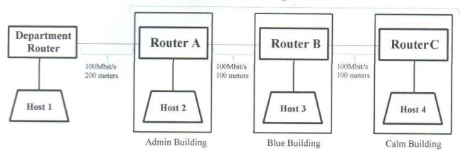
a) Using a diagram, illustrate how long a packet of length L bytes will take to travel over an idle network from Host 4 to Host 1? The routers use a store-and-forward architecture.
