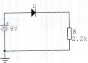
(ii) Suppose the diode in e(i) is reversed, determine  $V_D$ ,  $V_R$ , and  $I_D$ .
