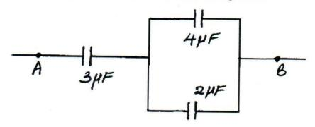
(i) Calculate the effective capacitance between **A** and **B**.(3 marks)
