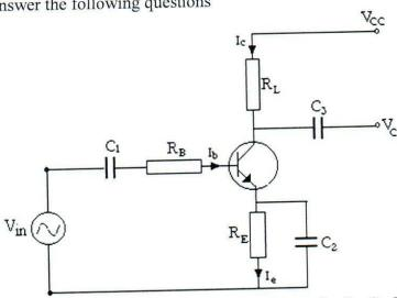
What is the function of each of the following circuit components: C<sub>1</sub>, C<sub>2</sub>, C<sub>3</sub>, R<sub>L</sub>, R<sub>B</sub>.
