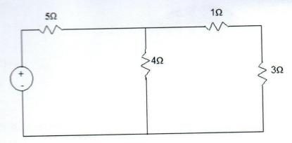
(i) Determine the Thevinin Voltage across the  $3\Omega$  resistor.
