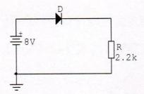
(ii) Suppose the diode in e(i) is reversed, determine V<sub>D</sub>, V<sub>R</sub>, and I<sub>D</sub>.
