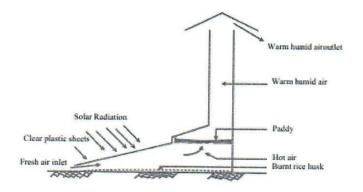
(i) Explain how the drying function is accomplished in the dryer shown
