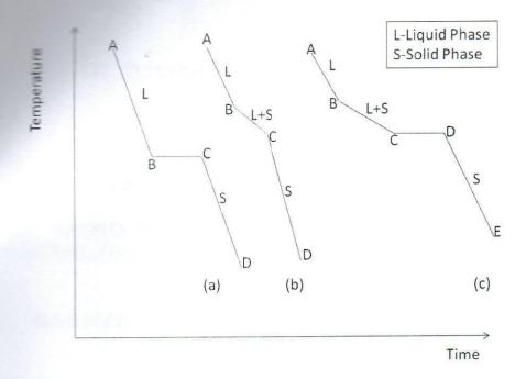
b) Discuss the effect of slow and rapid cooling curves with illustrations for a pure metal with reference to the concept of recalescence. (8 marks)
