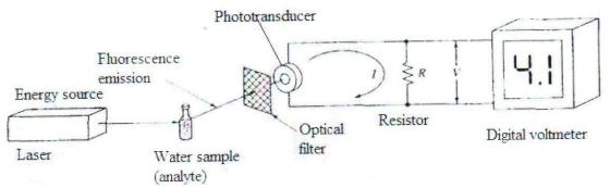
ii. A 25.0 ml sample containing Cu<sup>2+</sup> gave an instrument signal of 23.6 units (corrected for a blank). When exactly 0.5 ml of 0.0287M Cu(NO<sub>3</sub>)<sub>2</sub> was added to the solution, the signal increased to 37.9 units. Calculate the molar concentration of Cu<sup>2+</sup> assuming that the signal was directly proportional to the analyte.
