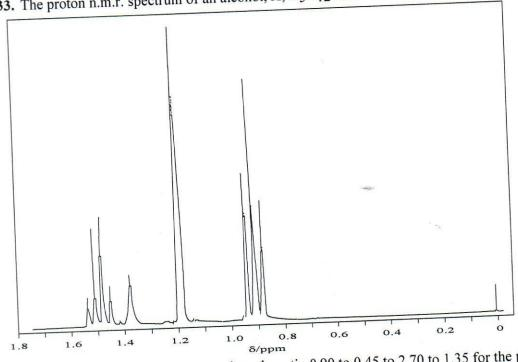
The measured integration trace gives the ratio 0.90 to 0.45 to 2.70 to 1.35 for the peaks at δ 1.52, 1.39, 1.21 and 0.93, respectively.
