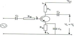
where  $R_B$ =1M $\Omega$ ,  $V_{BB}$ =30V,  $V_{CC}$ =30V,  $R_E$ =10K $\Omega$ ,  $R_C$ =5K $\Omega$  and  $\beta$ =100. Calculate  $I_e$ ,  $I_c$ ,  $I_b$ ,  $V_C$ ,  $V_E$  and  $V_{CE}$ .
