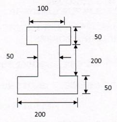
If the maximum bending stress in the beam section is not to exceed 40MPa. Find the moment, which the beam can resist. (20MKS)
