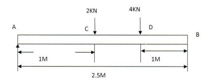
Draw the shear force and bending moment diagrams for the beam.
