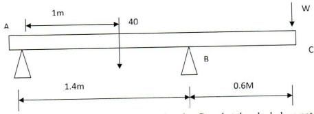
Find the maximum weight W, that can be placed at C so that the plank does not topple.
